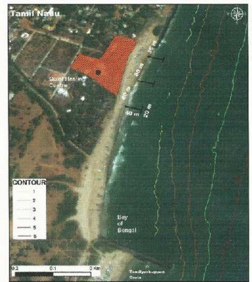
Conceptual layout of Proposed T-groynes
