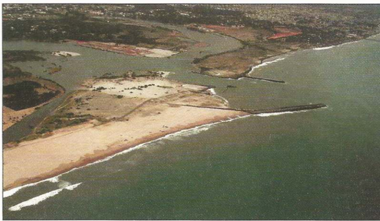
Sand has accumulated south of the Pondicherry harbour entrance, the beaches north have disappeared
