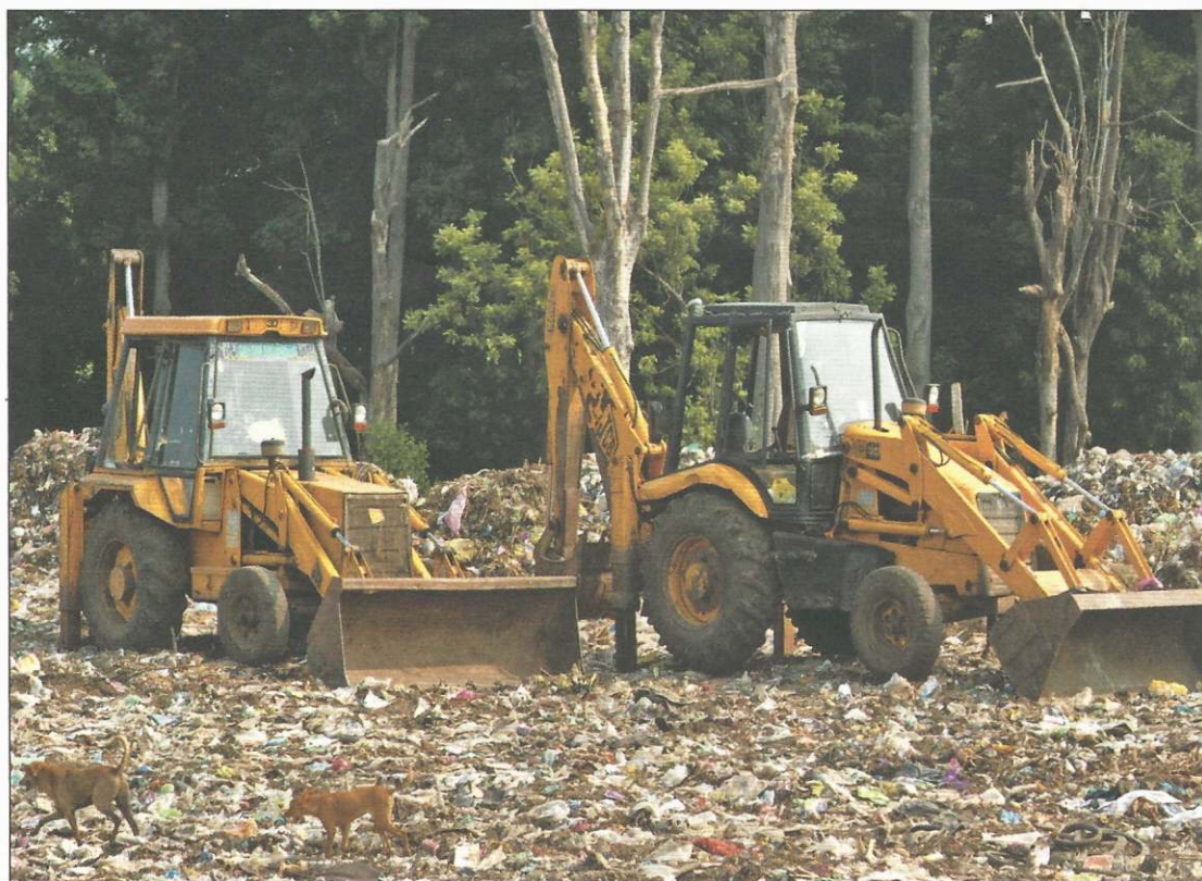
Excavators turn over the waste at the landfill every day to stop the production of methane
