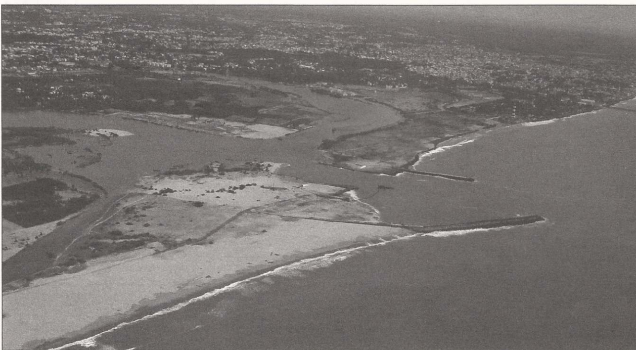
The breakwaters south of Puducherry that protect the Puducherry harbour. They have created a wide beautiful beach to the south, but have led to loss of entire beaches and even parts of coastal villages to the north.
