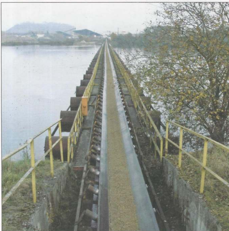
Excavated earth from the Matrimandir Lake can be moved by conveyor belt to create the hill for the upper lake. This photo shows a conveyor belt in Germany, transporting earth over water.
