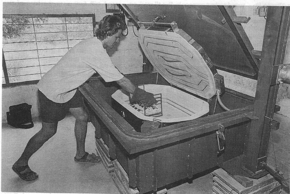
At the Matrimandir workshop: Placing the gold-glass sandwich tiles in the electric vacuum oven
