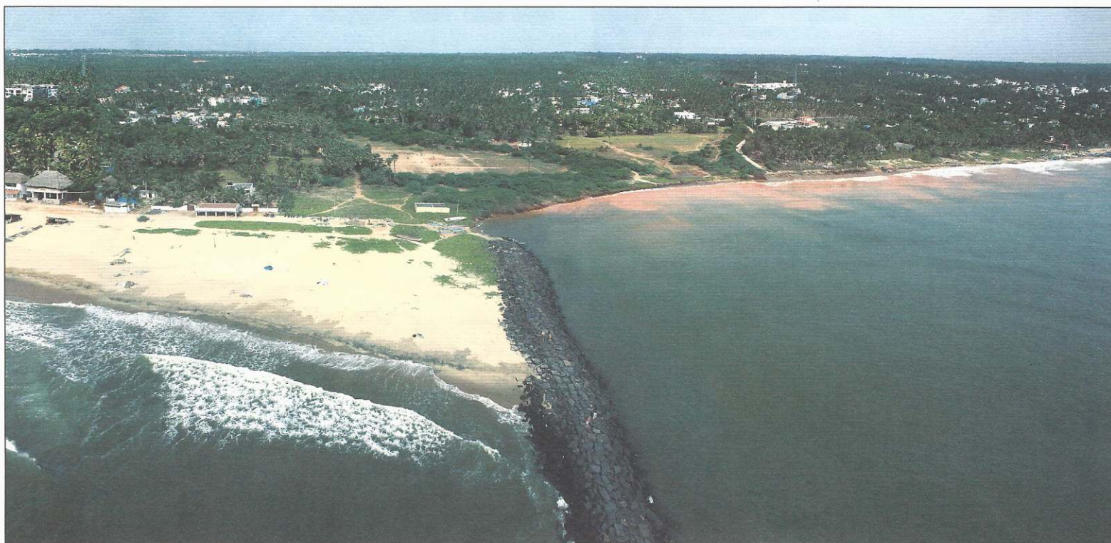
The disruption of littoral drift caused by the groyne at Thandirayankuppam, south of Quiet, causes beach accretion to the south and beach erosion to the north of the groyne. Aerial panoramic view, photo taken by kite on September 16, 2012
